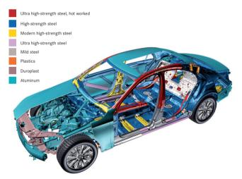
There are 8 different materials in your Mercedes-Benz that require specialised methods and equipment to join them together. Our fully dedicated team is trained to work with and repair such vehicular construction materials like aluminum alloys, magnesium alloys and ultra-high tensile steels.
